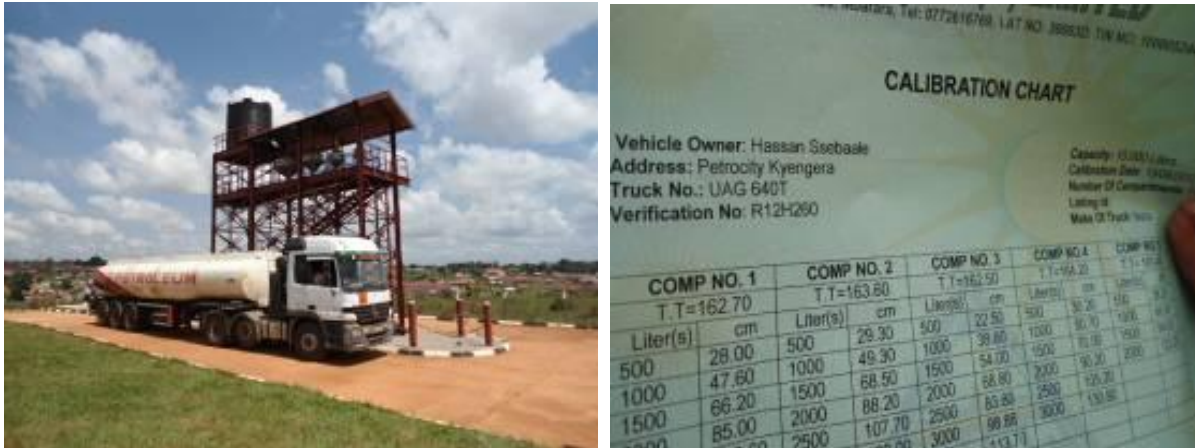
Calibration of fuel tank and a copy of results at UNBS Bweyogerere rig
