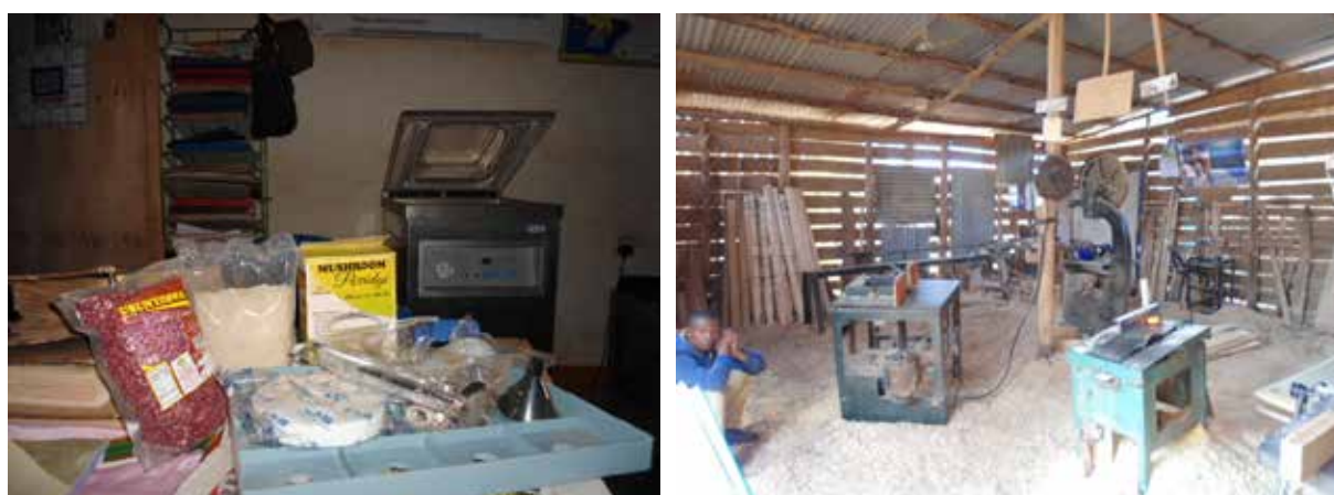
L-R: An automated vacuum sealing machine and some of the finished products at Lusaze and a wood drilling and mortise machine at Kijukizo Carpentry Hub in Butambala District
