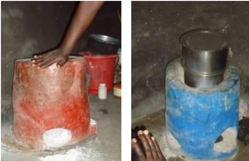
Energy saving stoves under use; beneficiary touches the stove to confirm that the stove remains cool even while cooking
