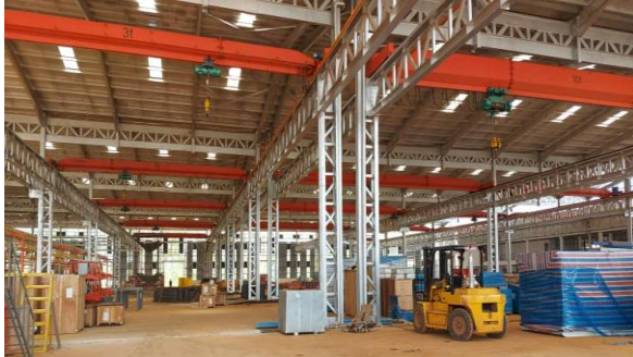
Left: The 3-ton and a 10-ton chassis crane; Right: Diesel and electric fork lifters at the Kiira Vehicle Plant in Jinja District
