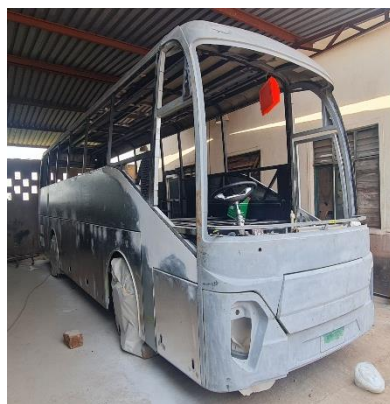
Left: Joining of panels to the bus chassis. Middle: Bus in the spray shop. Right: A bus nearing completion at Luweero Industries, Nakasongola District
