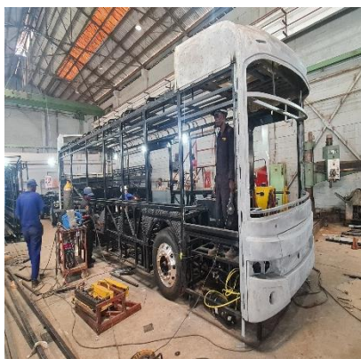
Left: Joining of panels to the bus chassis. Middle: Bus in the spray shop. Right: A bus nearing completion at Luweero Industries, Nakasongola District
