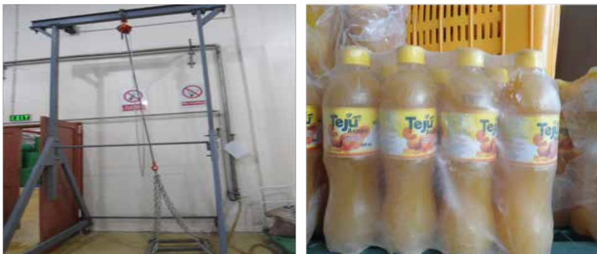
**L-R: Fabricated pulley system for offloading concentrate drums and finished mango RTD juice in PET bottles at Soroti Fruit Factory**
