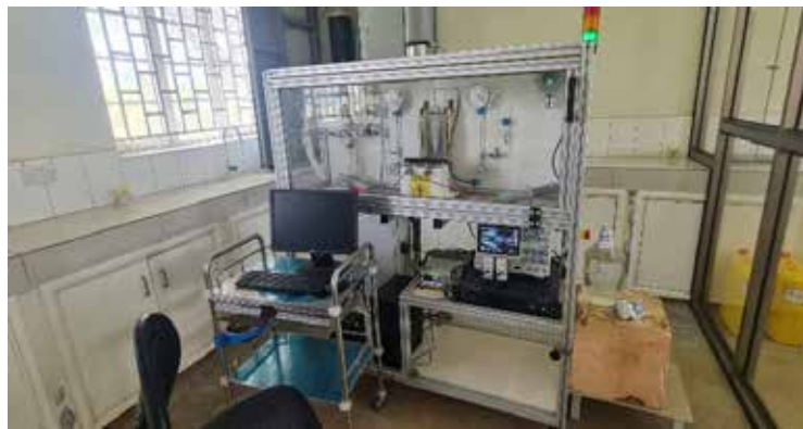
On site air-to-fertilizer mini-plant prototype installed in a laboratory at Kamenyamigo Satellite Station-MUZARDI in Lwengo District
