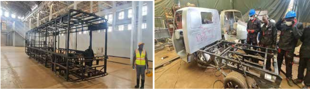
Left: The localized Kayoola EVS Frame at the KMC vehicle plant in Jinja. Right: Fabrication of the 3-in-1 Trike prototype at KMC office in Ntinda
